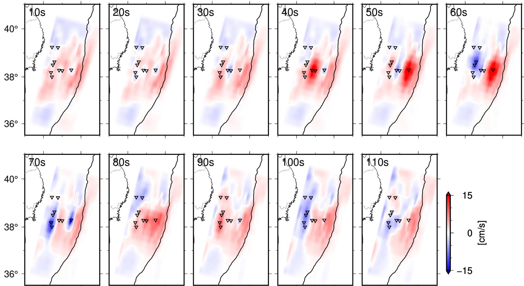
**Figure S3.** The temporal evolution of the seafloor displacement rate obtained by the inversion analysis.
