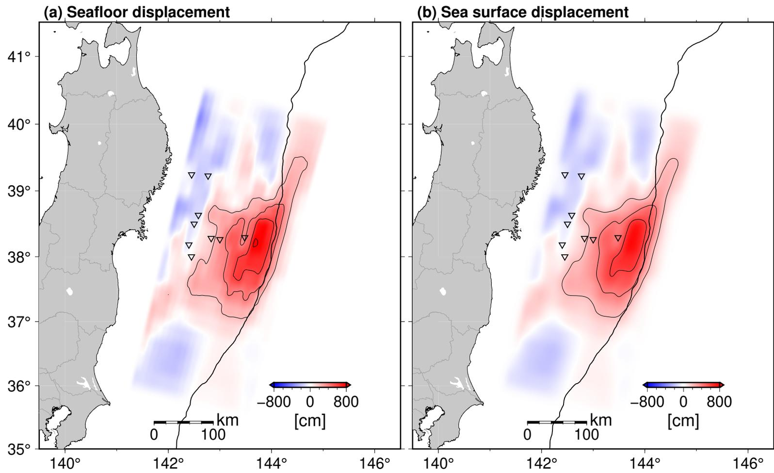
**Figure S2.** The spatial distribution of (a) the seafloor and (b) the sea-surface height obtained by the inversion analysis. The contour interval is 2 m.
