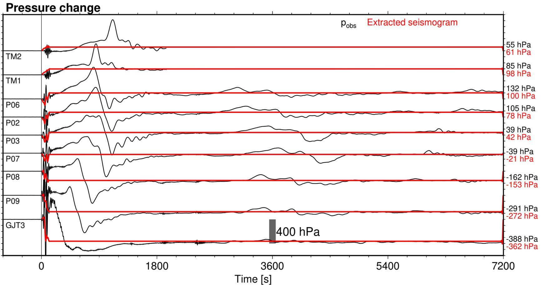
**Figure S5.** Comparison of the observed pressure time series (black) and those expected from the extracted displacement (red) for two hours from the origin time. The final pressure offsets, calculated by averaging the last 600 s time window, are also shown.
