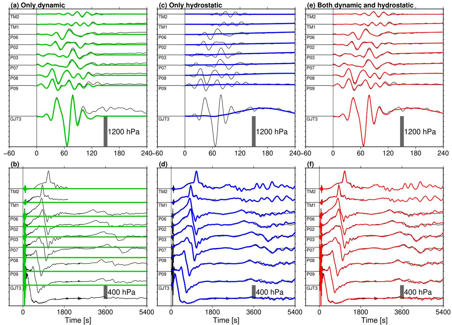
**Figure S1.** Comparison between the observed pressure waveforms (black) with the simulated waveforms, for (a,b) dynamic (green), (c, d) hydrostatic (blue), and (e,f) both pressure changes. The lowpass filter with a cutoff of 0.05 Hz is applied.
