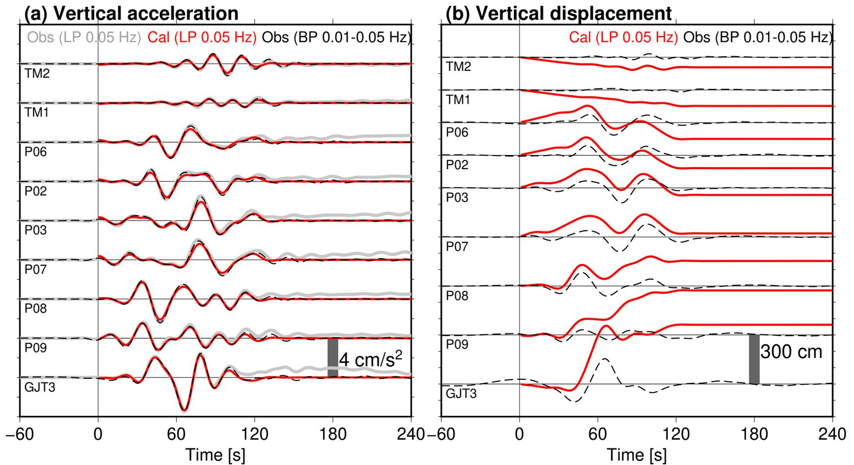
**Figure S6.** Comparison between the extracted seismograms (red), and the lowpass-filtered (0.05 Hz, gray) and the bandpass-filtered (0.01–0.05 Hz, black dashed) waveforms, for (a) vertical acceleration and (b) vertical displacement.
