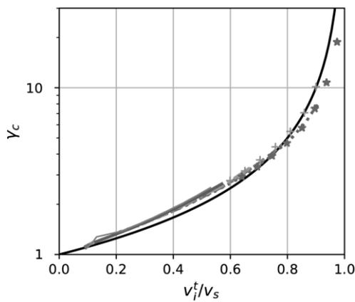
**Figure 1. Critical ratio  $\gamma_c$  plotted against rupture velocity  $v_i$  prior to cascading process. Black Solid line indicates analytical approximation and others indicate results of numerical simulation in various parameter settings.  $v_s$  is shear wave velocity.**
