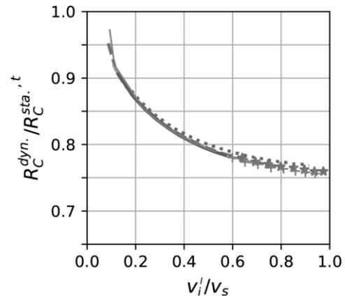
**Figure 2. Ratio of  $R_C^{\text{dyn},t}/R_C^{\text{sta},t}$  plotted against rupture velocity  $v_i$  prior to cascading process. Different symbols denote the results of different parameter settings.**
